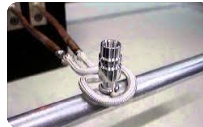
Induction Brazing for FT line Zero Emission
